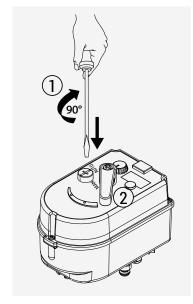
In the case of power failure or for service purposes, user can manually operate with the actuator:
