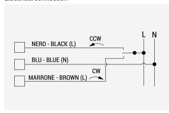
**A** WARNING. Make sure the power supply voltage is disconnected while the connections are being carried out.
