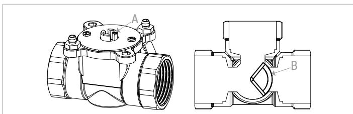
The valve rotor can turn by 90° in both directions (clockwise and anticlockwise); therefore, based on the initial point setting, it can move within a range of ±90°.
