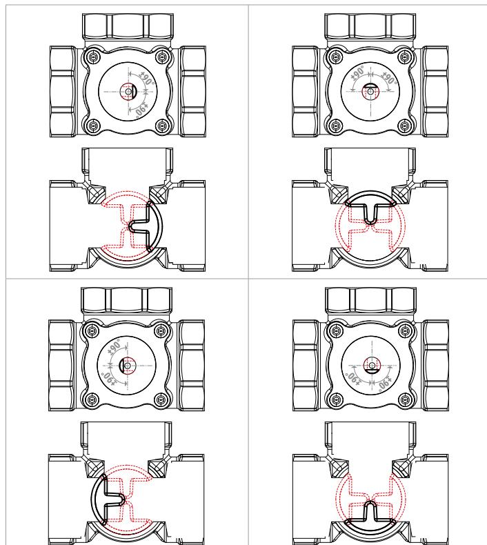
Set the correct operation values of the actuator (rotation direction, control signal, etc...) based on the desired rotor rotation, by using the internal DIP Switches.
