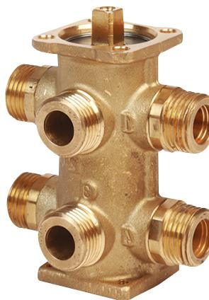
The R274C compact 6-way zone valve can control the water supply from two different thermal energy sources to a single usage point, in other words it controls 4-pipe systems (typically heating and cooling) in a simple way.
