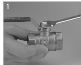
1 Remove the nut with the proper wrench
