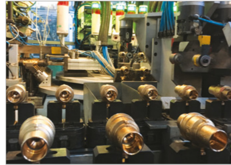
Automatic assembly with 100% in-line tests'
