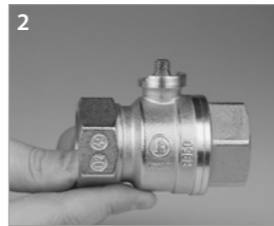
2 Remove the lever and insert the new PTFE stuffing box ring (included in the package) without removing the preassembled one
