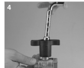
4 Tighten the nut completely using the proper socket wrench
