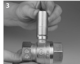
3 Install the cylindrical extension placing it on the ball valve rod and paying attention to the opening direction
