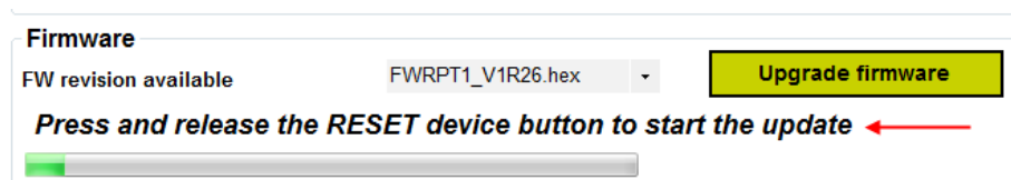
Figure 46 - GE552Y053 firmware update indications
