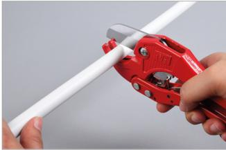
Cut the pipe 90° to its axis with a cutter (we recommend turning the cutter slightly during this operation) or a roller pipe cutter to prevent ovalizations.
