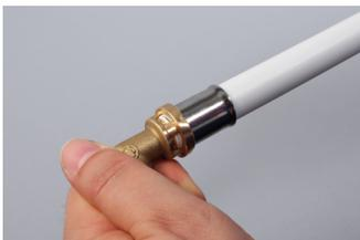
Insert the pipe all the way inside the fitting; the correct coupling position of the pipe can be checked visually through the bush ring slots. The bush flared profile makes the insertion easier.
