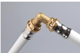
Verify proper fitting by looking at the bush ring to verify the correct position of the pipe. This is a one-time operation, in case of improper pressing the pipe must be cut and a new fitting is required to create the joint.
