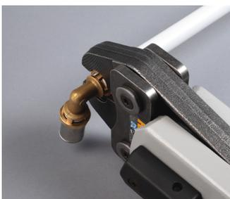
To press the fittings, use a jaw of the same size of the fitting and profile complying with table "Jaws profiles" on page 2:
