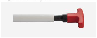
**3)** Insert the pipe up to the stop on the fitting. For  $\emptyset$  20: insertion force =  $6 \div 16$  kg
