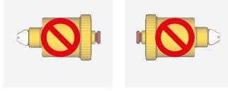
▲ WARNING. Close the cap of the air vent valve when rinsing out and filling the system, to prevent impurities from entering the mechanisms of the valve and damaging it.
