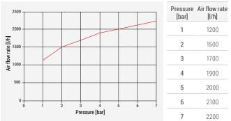
**NOTE.** The air discharge capacities of the R99 valve increase progressively at the pressure increase by showing the efficiency of the mechanism.
