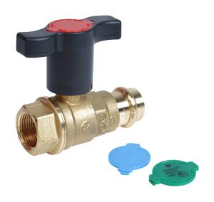
Ball valve, with female threaded-press connections (for copper pipe complying with EN 1057; for stainless steel pipe complying with EN 10217-7 and EN 10312; for carbon steel pipe complying with EN 10305-3), for pipes with high insulation thickness, specific for domestic water. Full port.
