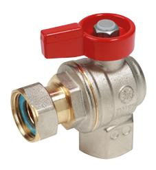
Angle ball valve, with female-female threaded connections with nut and gasket, specific for under boiler use and for meters connection.
