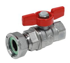
Ball valve, with female-female threaded connections with nut and gasket, with adjustable tail piece (valve length adjustment: 8 mm), specific for meters connection. Full port.
