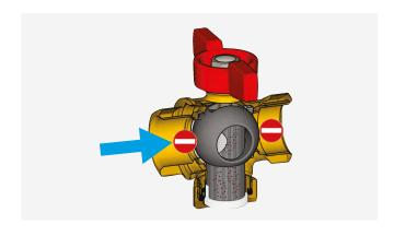
When the valve is closed the heat transfer fluid cannot flow through the filter as this is isolated from the rest of the hydraulic circuit.
