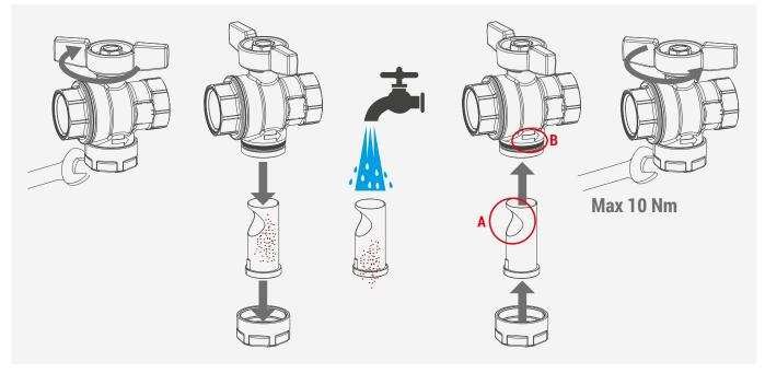
**A WARNING.** After filling the system, we recommend cleaning the filter for the first time after a week of use to remove any obstruction caused by installation residues (metallic chips, seal elements.)
