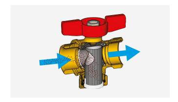
When the valve is open the heat transfer fluid flows through the filter, then it slows down to enable the separation of solid debris.
