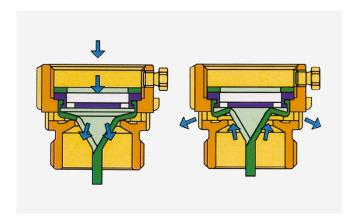
The R622 backflow preventer is directly screwed onto the cock before the swivel that is attached to the hose barb.
