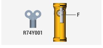
Manual air vent valve mounted on delivery manifold. It must be moved using the special R74Y001 wrench. For proper operation, a dearetor filter **F** has also been installed inside the support insert and can be easily removed for replacement or ordinary maintenance operations.
