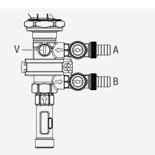
A mechanical flow meter connected to the KTD regulation unit reads the flow. The **V** valve adjusts the flow starting from the "completely open" position (screwdriver tip in vertical position) and turning clockwise.
