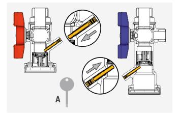
The ball valves integrated in the circulation unit for sectioning of the solar panels are both equipped with a check valve to prevent undesired circulations.
