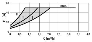
Recommended for two-pipe heating systems with radiators to reduce the flow noise at thermostatic valves. The pump reduces the delivery head to half in the case of decreasing volume flow in the pipe network.
