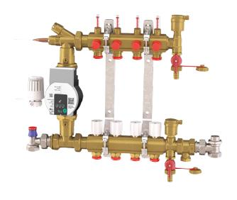
R557F-1 manifold is used in those applications where in the same housing unit, are installed heat sources supplied at high temperature water and radiant panel circuits to be supplied with low temperature water.
