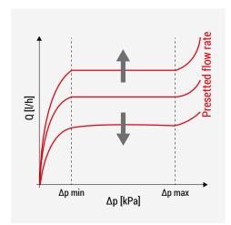
Manifolds with dynamic flow balancing are used primarily in radiant systems.
