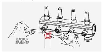
To connect the system circuit pipes use suitable adaptors for copper, plastic or multilayer pipes from the R178E, R179E series.
