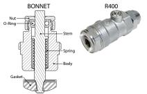
The bonnet replacement with R400 key, is not possible for the following valves: R401DX004, R402DX004
