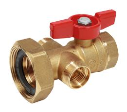
Ball valve, with female-female nut threaded connections, specific for circulator connection, with additional connections for thermometers or other optional components.
