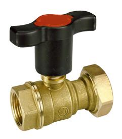
Ball valve, with female threaded connection-nut female, with integrated check valve, specific for circulator connection, for pipes with high insulation thickness. Standard port.
