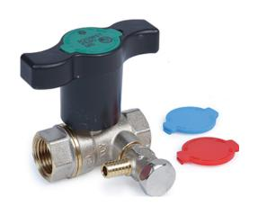
Ball valve, female-female connections, with drain cock with hose connection  $\emptyset$  9 mm, for pipes with high insulation thickness, specific for domestic water. Standard port.
