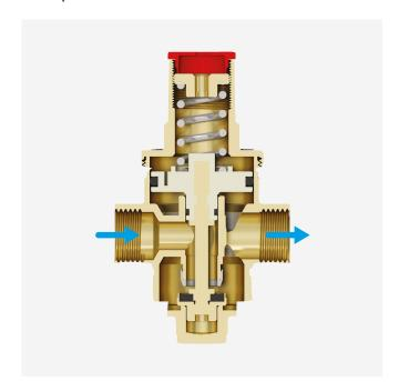
A piston actuates the stopper movement, as consequence from the two opposing forces: water pressure from the bottom in the pipe downstream from the reducer (which tends to close the valve), pushing from the top by an appropriately loaded spring in relation to the work pressure in play (tends to open the valve).
