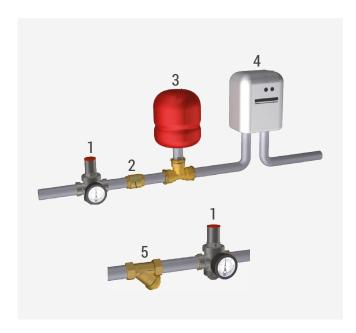
We recommend to install a filter before the reducer to eliminate all impurities in the water that may deposit onto the reducer seat and cause malfunctions.
