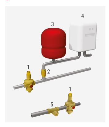
We recommend to install a filter before the reducer to eliminate all impurities in the water that may deposit onto the reducer seat and cause malfunctions.
