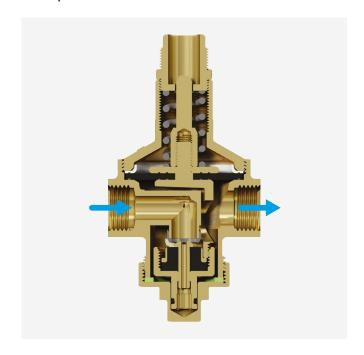
A flexible diaphragm actuates the stopper movement, as consequence from the two opposing forces: water pressure from the bottom in the pipe downstream from the reducer (which tends to close the valve), pushing from the top by an appropriately loaded spring in relation to the work pressure in play (tends to open the valve).
