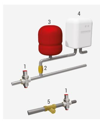
We recommend to install a filter before the reducer to eliminate all impurities in the water that may deposit onto the reducer seat and cause malfunctions.
