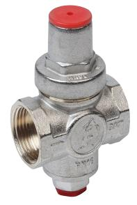
The R153C pressure reducer is an automatic valve that reduces and stabilizes the pressure of a fluid in a water distribution conduit according to a preset value.
