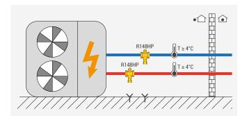
When the water temperature drops down to 1 °C, the valve opens and drain the pipe to prevent freezing.
