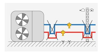
Freezing protection valves must be installed:
