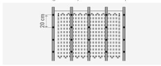
Ceiling installation of a radiant system requires the creation of a supporting structure in the false ceiling
