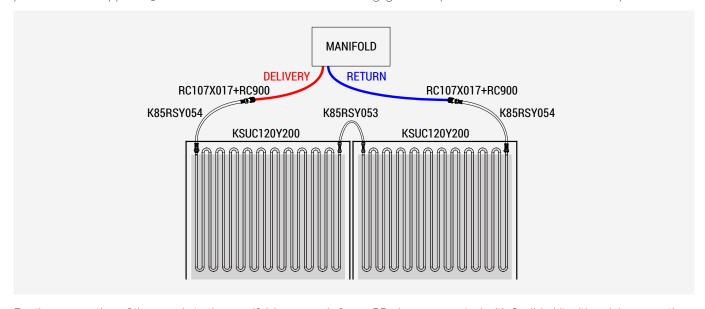
For the connection of the panels to the manifold, are used 16 mm PB pipes connected with flexible kit with quick connections of the K85RS series via RC107X017 brass fitting with RC900 sleeves.
