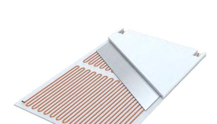
The panels of the GKC Ultra-C series, designed for the installation of heating and cooling radiant ceiling systems, consist in a plasterboard with graphite, an aluminum foil, a thermal activation composed by one circuit with 12 mm copper pipe and a sintered expanded polystyrene (EPS150) insulating layer, for a total thickness of 40 mm.
