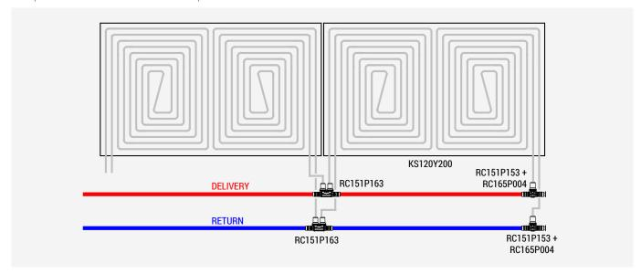
Panels should be connected using multilayer pipes  $\emptyset$  20 x 2 mm that have not been pre-insulated (in bars) or pre-insulated (in coils) and RC-P series plastic push-fittings.
