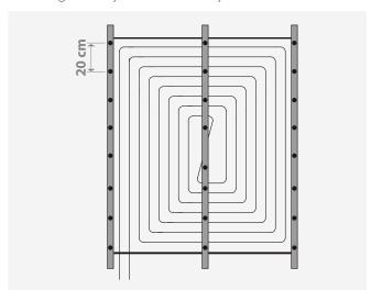
Ceiling installation of a radiant system requires the creation of a supporting structure either in the false ceiling or against the ceiling.
