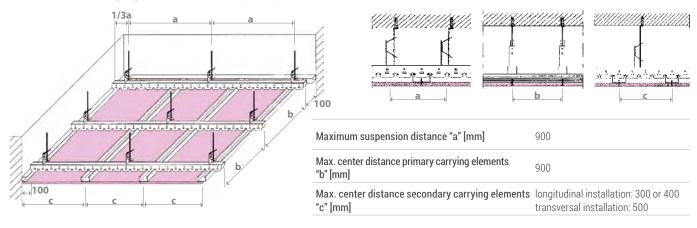
Especially for compact installations, a clearance of approx. 25÷50 cm can be left between panel rows to insert backbone links. Moreover, the pipes coming out of individual radiant panels should be installed over risers, to prevent crushing.
