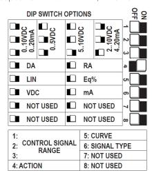
**DIP SWITCHES 1, 2, 3** are used to change the analogic inlet ranges. To change from a voltage analogic inlet to an analogic plug, set **DIP SWITCH 6** on the desired position.
