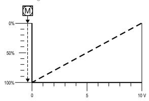
**DIP SWITCH 5** enables to change the control feature of the actuator to obtain a linear combination of the valve and the actuator or an almost identical percentage.
